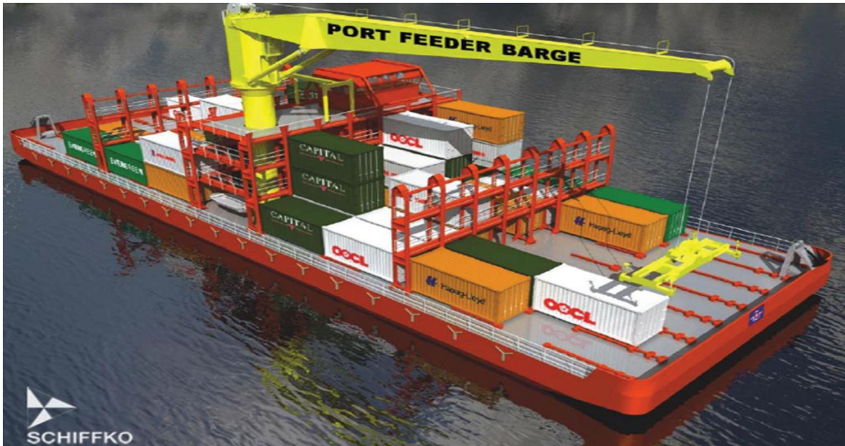
Figure 9 Floating Barge Crane
